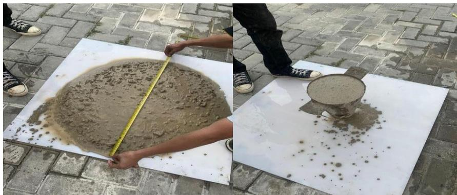
**Gambar 4.** Pengujian *flowability*
